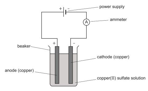
Which reaction occurs at the anode and which reaction occurs at the cathode for this experiment?
